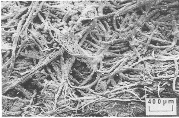
Figure 5 SEM of edge of fibre-cement-silica sheet containing curled fibres.
